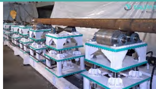
Workpiece Handling System Rear Side - Hydraulic Steady Rest - 5 Nos. Rear Side - Hydraulic Jack - 5 Nos.
